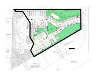
Phase 1 of the parking hub project provides 33 new parking spots in the downtown core. Construction will include drainage and storm pipe connections, relocating and servicing of the Tugwell Fields washroom, installation of electric vehicle charging stations, and access pathways. Phase 2 of the project will be considered in the future depending on demand.
